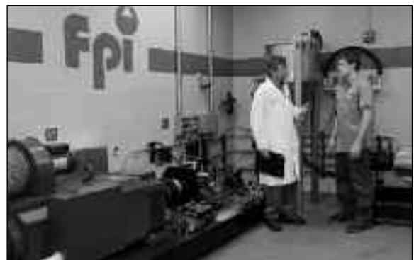
Caption 200 HP dynamometer with electrical regeneration capabilities used for testing the energy efficient fluids.
